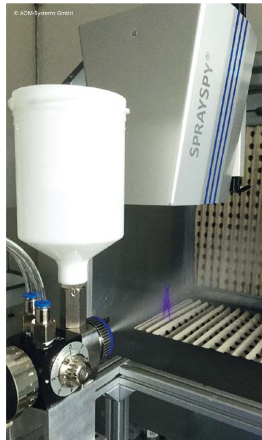
The laser light detects even the smallest deviations from the setpoint in the spray jet.
