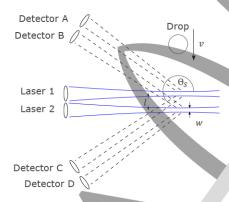
TOF: Time difference between the signal at detector A and detector B. The same holds for detector C and detector D.
