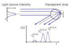
Scattering light from transparent particles can be interpreted as the superposition of all scattering orders present at the detector location:
