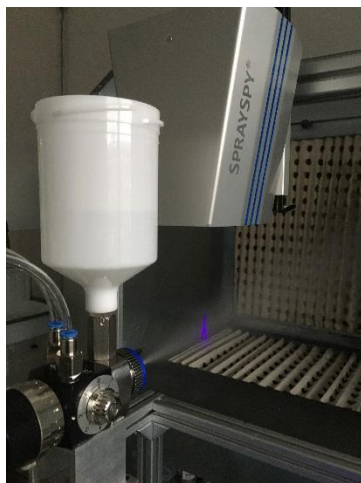
The laser light in the spray detects even the smallest deviations from the target value.
