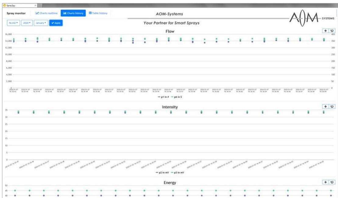
Screenshot from the database: Online and in real time, the user can follow the measurement on the Internet.
