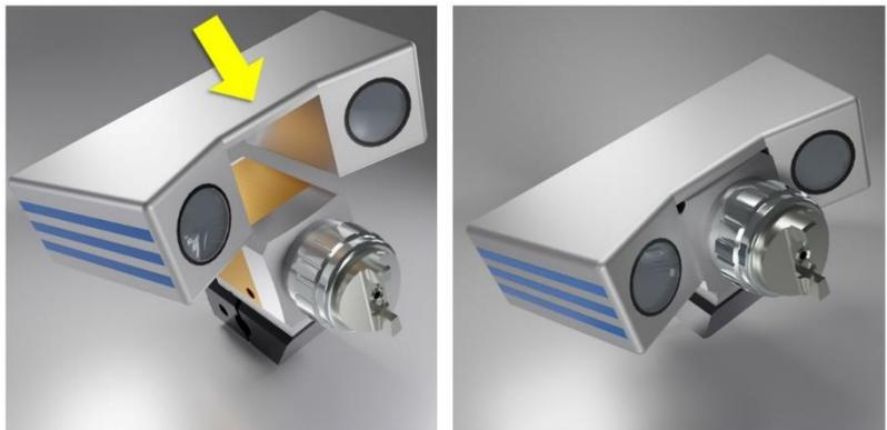
*The latest generation "SpraySpy" is placed directly on the gun and measures the spray in use.*
