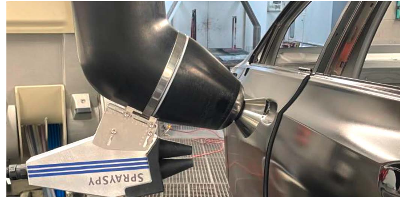
The 'SpraySpy' measuring system monitors the paint in the spray jet and makes it possible to predict the final coating thickness. Photo: Volkswagen
