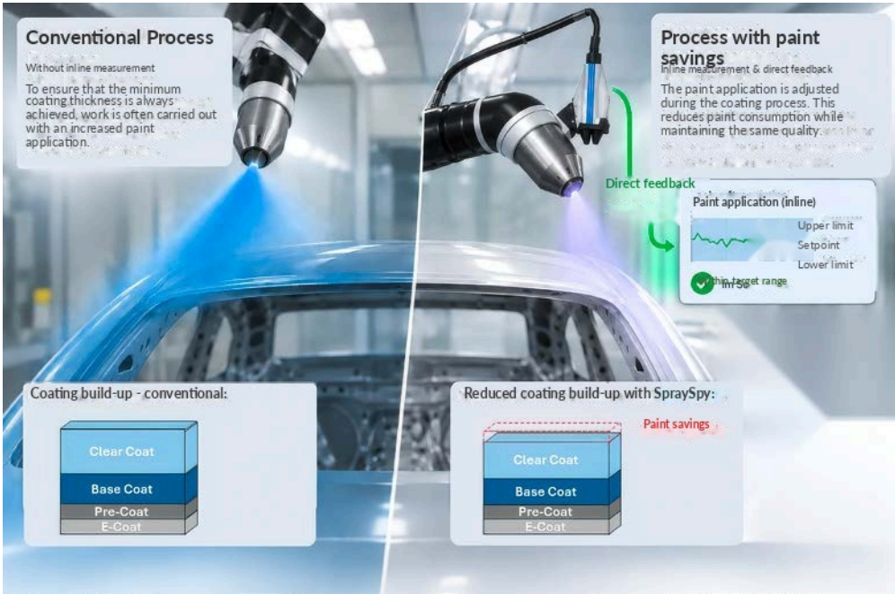
The comparison shows the difference between the conventional process and the process with paint savings.
